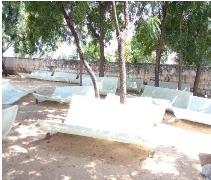
Figure 4. 11 Multiple GRP panels after curing
