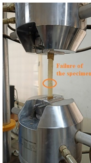
Figure 4. 18 Tensile test of the three-layered GRP specimen
