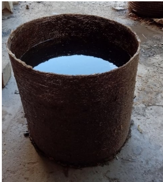
Figure 4. 3 Water filled after curing
