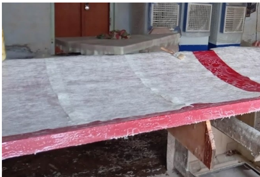
Figure 4. 9 Application of bi-directional glass fibre mats on dye frame along epoxy resin-hardener mix coat
