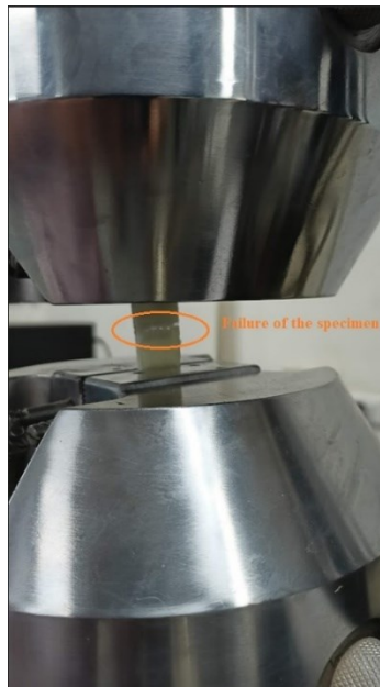
Figure 4. 22 Compressive strength test of two-layered GRP specimen
