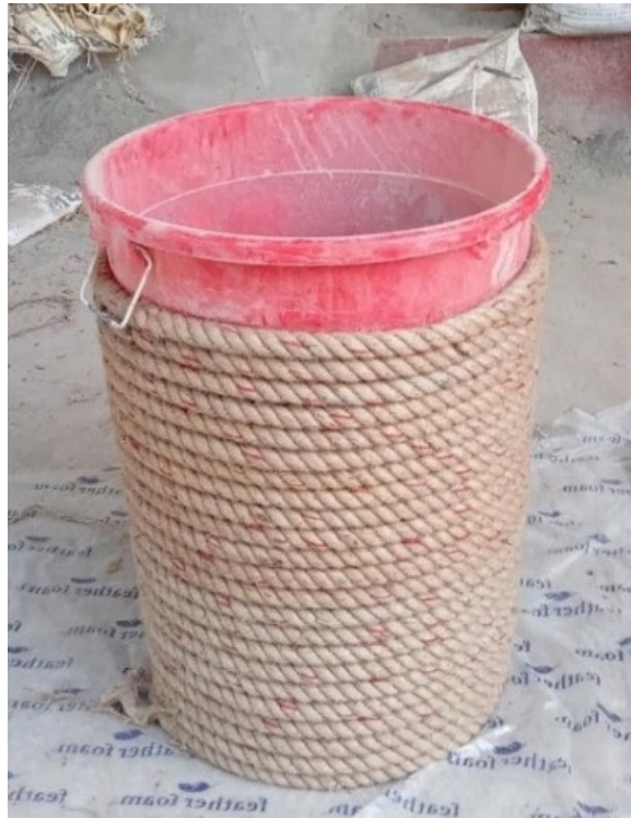
Figure 4. 4 Winding jute fibre to the mould
