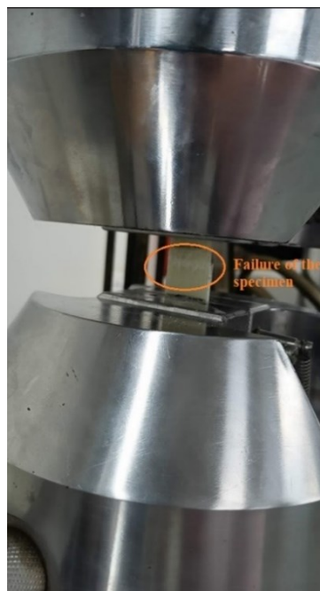
Figure 4. 23 Compressive strength test of three-layered GRP specimen
