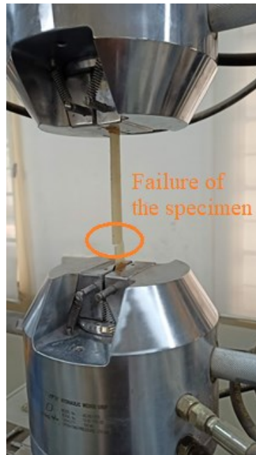
Figure 4. 14 Tensile test of the two-layered GRP specimen
