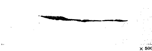
Fig. 44b. Longitudinal view of duplex silicate-sulphide inclusion in hot-rolled steel. Unetched. (Boulger, Battelle)
