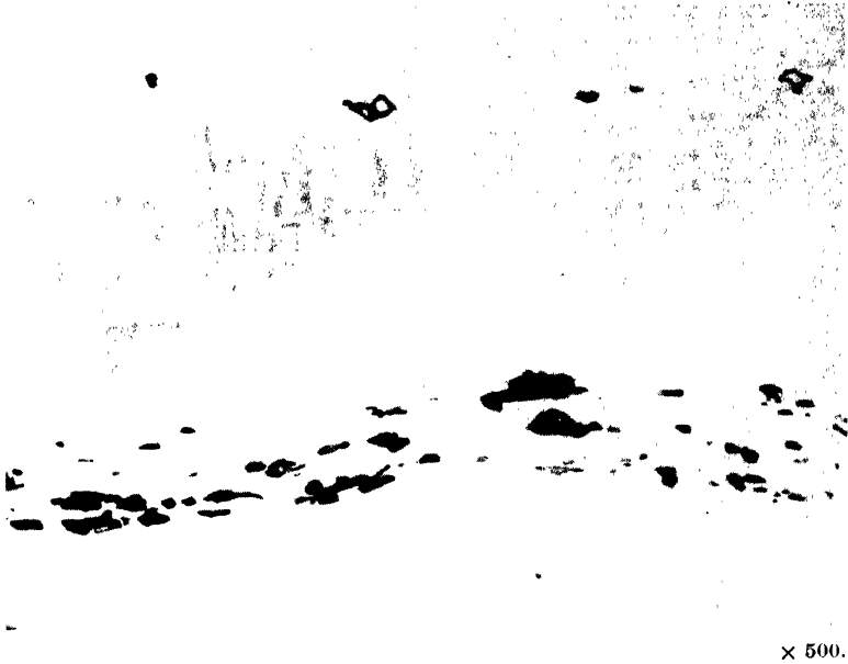
FIG. 46. Same as Fig. 45 but at higher magnification. Note the sharp corners on the inclusion in the upper center. Unetched. (Fick, Battelle)
