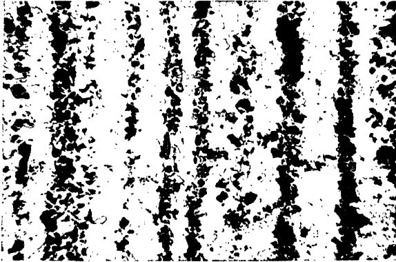
Fig. 52a. Banded structure, after furnace cooling from 1600°. Note sulphide inclusions, elongated in the rolling direction, above arrow.
