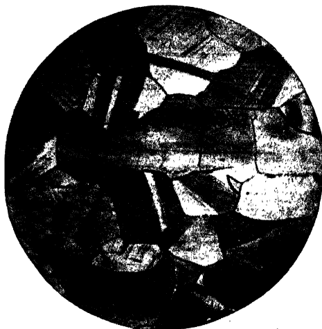
FIG. 16. Rolled manganese steel water quenched from 1925^{\circ} . \times 100 . (Battelle) 1.36 C, 0.36 Si, 14.20% Mn.
