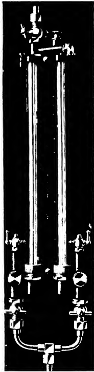
FIG. 56. The Amal flowmeter, Mark VIII type. [See page 103.]
