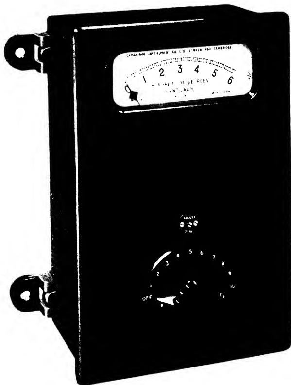
FIG. 317 -The Cambridge exhaust temperature indicator
