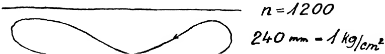
FIG. 203.—Suction diagram taken from carburettor choke tube of four-stroke engine at 1200 r.p.m.
