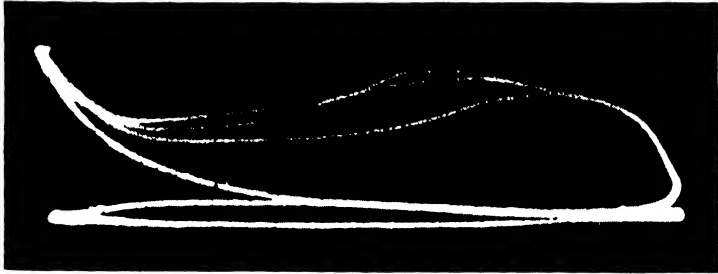
FIG. 263. Indicator diagram taken with ignition fully retarded, 1200 r.p.m.
