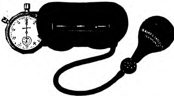
FIG. 352.—The recording pattern Whidbourne stroboscope.
