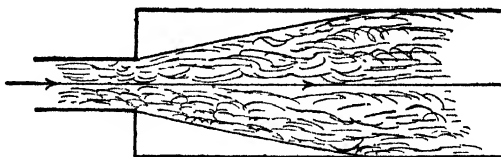
FIG. 278.—Expansion of a fluid from a small into a large section.
