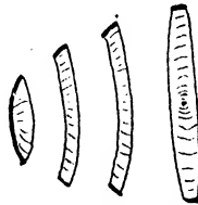
Fig. 10.—Sketch to show how Boards shrink.
