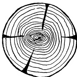
Fig. 3.—Log with Starshakes.
