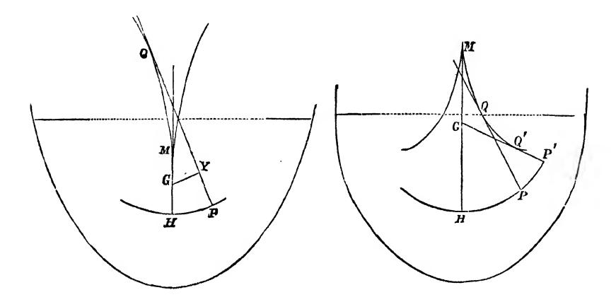
assumed that the ship can be divided symmetrically by a plane perpendicular to its length, and in this case the ship has two vertical planes of symmetry, and consequently the vertical line HG passes through the centroid of the plane of flotation.
