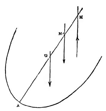
Taking moments about G, the centre of mass of the vessel, the resultant fluid pressures will tend to restore equilibrium, or the reverse, according as
