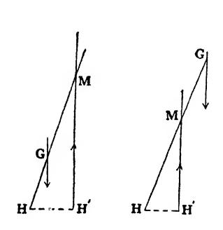
When this condition is satisfied the vertical through H' intersects the line HG in a point M called the **metacentre.** The couple acting on the body is W.  $GM\theta$ , and it tends to restore the body to its former position or to increase the displacement according as M is above or below G.
