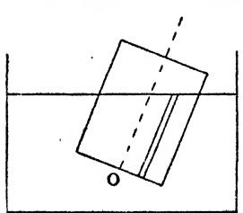
Take the origin O at the centroid of the base of the floating cylinder, which is of area A. Let the plane of the surface of the liquid be
