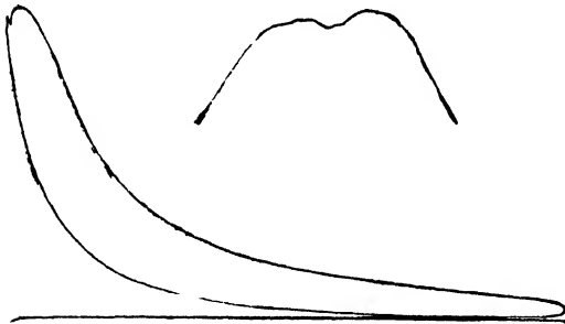
Fig. 12.—DIAGRAM SHOWING LATE FUEL INJECTION Compare with Fig. 6.
