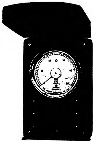
FIG. 296.—MINIATURE CIRCULAR SCALE COMBINED TESTING SET. (Record Electrical Co., Ltd.)
