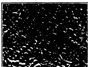
FIG. 1.—Surface of cast copper, 30 diameters.
