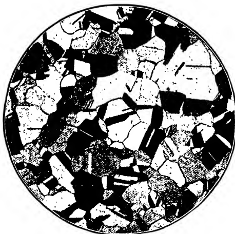
FIG. 28.—Brass which worked satisfactorily. X 100.
