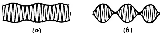
FIG. 82.—The amount by which the modulation causes the amplitude of the carrier to vary depends upon the loudness or softness of the sound.
