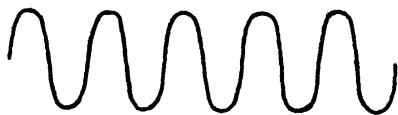
FIG. 32.—The current fluctuations in the output of the photo-electric cell produced by the scan of one line of Fig. 31.
