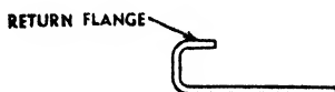
FIG. 44.—A return flange adds still greater stiffness than one involving (as in Fig. 43) only a single bend.
