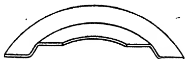
FIG. 39.—A flange thrown up around a lightening hole adds greatly to stiffness.
