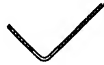
FIG. 57.—Notching or piercing after forming, as here indicated, tends to avoid distortion of the piece and of the hole or notch.
