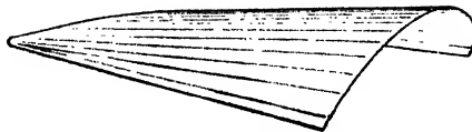
FIG. 51.—Wing leading edge formed in a die such as that shown in section in Fig. 50.
