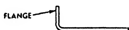
FIG. 43.—A flange formed at the edge of a stamping stiffens it materially.
