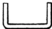
FIG. 20.—An inside radius less than stock thickness or a sharp square corner, though sometimes feasible, should be avoided.
