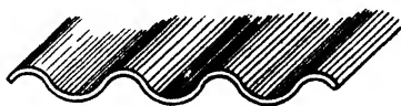
FIG. 40.—Corrugations add greatly to stiffness or resistance to bending across, but not to bending parallel to the corrugations.
