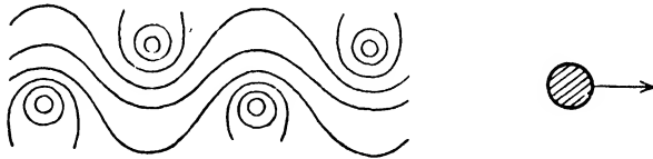
FIG. 22.—THE STRONGLY EDDYING WAKE CAUSED BY A CIRCULAR CYLINDER AT ORDINARY SIZES AND SPEEDS.
