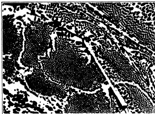
FIG. 106. Special hypereutectic cast iron, showing primary cementite and ledeburite eutectic. Carbon about 4.5%. Not a typical white cast iron because it contains an excess of carbon as \text{Fe}_3\text{C} . \times 100 .
