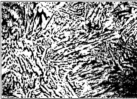
FIG. 114. Brass. Muntz Metal, 60% Cu-40% Zn, as cast. Etchant: Rosenhain's reagent. Showing Widmanstätten structure resulting from \alpha (light) separating from \beta along certain crystallographic planes. Final structure is \alpha light + \beta' (dark). \times 100 .
