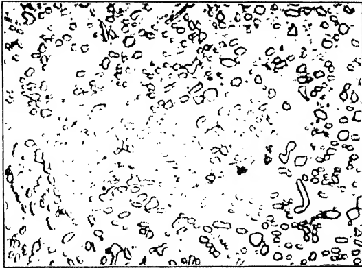
FIG. 72. Spheroidized carbide produced by very slow cooling of a previously normalized 1.00% C steel. Cooled from 1400 to 1200°F in 10 hr. \times 1000 .
