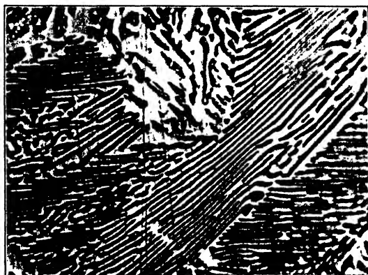
FIG. 116. Bronzite. Eutectoid structure of Cu-Sn system. Cast alloy having composition Cu 73%-Sn 27%. Reaction is \beta - \alpha + \delta . \alpha (light) is the matrix with \delta (dark) in relief. This structure is called bronzite because it strongly resembles lamellar pearlite in Fe-Fe 3 C system. \times 1000 .
