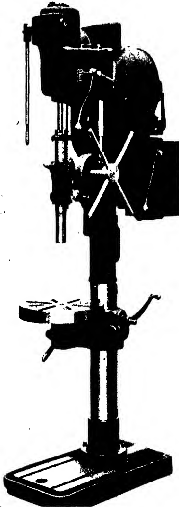
FIG. 98.—Vertical drilling machine with individual motor drive. ( Courtesy of The Cincinnati Bickford Tool Company. )
