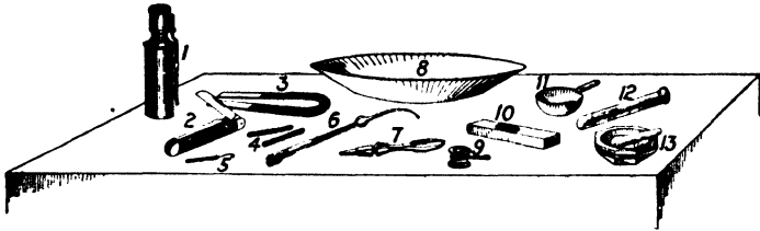
FIG. 22.—A blowpipe outfit. (1) Torch for blowpipe; (2) knife; (3) magnet; (4) glass tubes for platinum loop (5); (6) blowpipe; (7) forceps; (8) pan; (9) lens; (10) charcoal for blowpipe; (11) porcelain dish; (12) test-tube; (13) agate mortar for grinding small pieces of rock.
