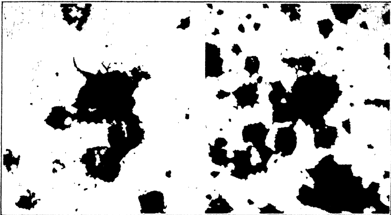
FIG. 99.—Zinc Sprayed on to Cold Glass. \times 50 .
