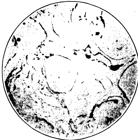
Fig. 130.—Surface Appearance of a Sprayed Metal, Aluminium-sprayed Iron (Arnold). \times 250 .
