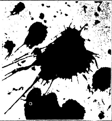
FIG. 102.—Aluminium Sprayed on to Glass Heated to 400^{\circ}\text{C} . \times 50 .
