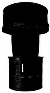
Fig. 228.—Power Cylinder Showing Exhaust Ports Cast Integral with the Cylinder Barrel. The Large Area for Water Jacket and the Mounting Flange, Bethlehem Engine
