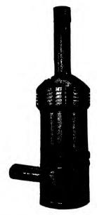
Fig. 260.-Air Compressor Piston, with Wrist Pin Partly Withdrawn
