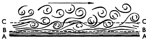
FIG. 22. Change from streamline to turbulent flow between pipe wall and axis.
