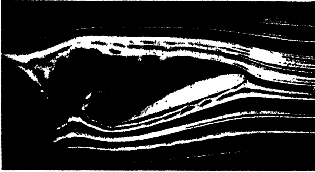
Separation occurring on an airfoil at a high angle of attack.
