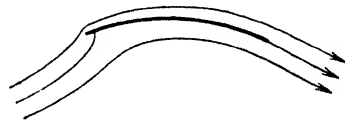
FIG. 140.—Flow round circular arc with such circulation that rear edge is left smoothly.
