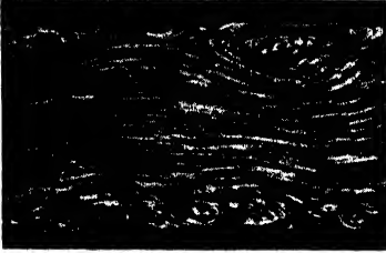
FIG. 39.—Turbulent flow in an open channel; the speed of the camera is about equal to the speed of the water near the walls.
