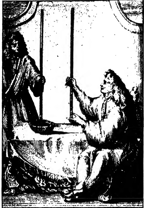
FIG. 102. AN EARLY ILLUSTRATION OF THE CONSTRUCTION AND USE OF A TORRICELLI TUBE (Courtesy of Taylor Instrument Companies.)
