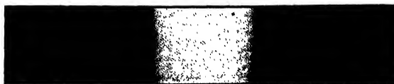
FIG. 305. APPEARANCE OF DIFFRACTION PATTERN PRODUCED BY PASSAGE OF LIGHT THROUGH A SLIT (From Studies on Optics , by A. A. Michelson. The University of Chicago Press, publishers.)
