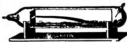
Fig. 319. DEFLECTION OF CATHODE RAYS BY A MAGNET.
