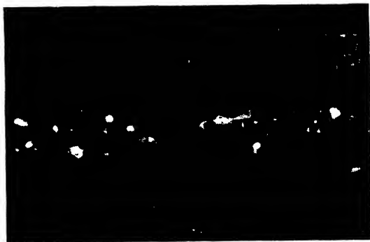
FIG. 322. --X-RAY PHOTOGRAPHS OF BUTT WELDS IN MILD STEEL.
