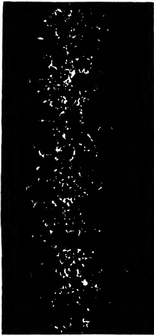
FIG. 336.---PHOTOGRAPH SHOWING TRACK OF A BEAM OF X-RAYS IN AIR.
