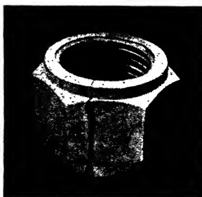
FIG. 131.—Season crack in a cold-worked brass fitting which had been exposed to ammonia fumes. Composition: copper 60, zinc 40. (Courtesy Professor C. Upthegrove.)
