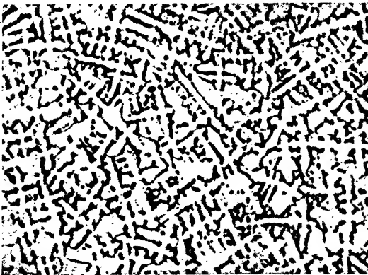
FIG. 104.—Microscopic structure of alpha brass (70 Cu, 30 Zn) when cast in sand. \times 100 . This shows the dendritic structure due to rapid cooling.
