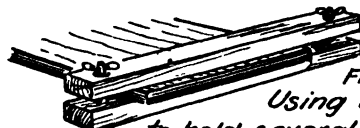
Fig 357. Trimming away surplus veneer after gluing.
