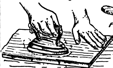
Hot Iron used to remelt the glue after laying and damping the veneer Fig 362.
