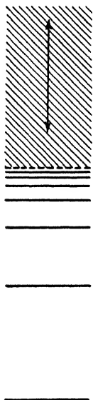
FIG. 62. Transitions corresponding to the electron retardation continuum represented in the energy-level diagram of an atom.
