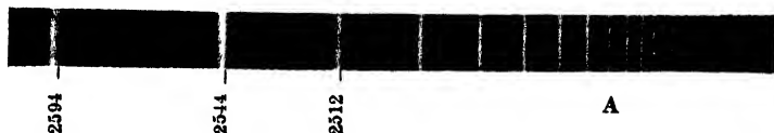
FIG. 41. Spectral line series of the sodium atom absorbed by sodium vapor. (After H. Kuhn.)
