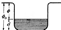
FIG. 208. Potential-well model of a metal. \Phi = effective work function, \phi_0 = work function for electrons in the lowest energy state of the conduction band, \delta = Fermi surface = zero-point energy of the electrons in the highest occupied electron levels.
