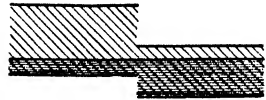
FIG. 206. Overlapping of the highest occupied energy bands of a bivalent metal and occupation of the two bands by electrons. For clarity the two bands are shown side by side.
