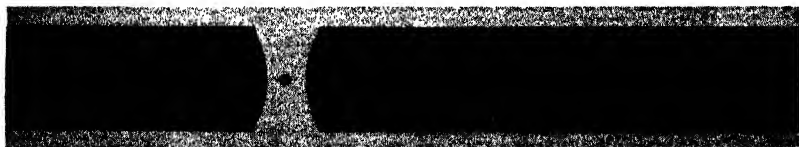
FIG. 37. X-ray diffraction pattern of CeO_2 crystal powder taken with method illustrated in Fig. 36.
