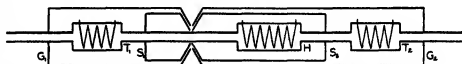
FIG. 6 Osborne-Stimson-Sligh flow calorimeter for specific heats of gases. T_1 , T_2 , inlet and outlet resistance thermometers, H , heater, S_1 , S_2 , shields in thermal contact with gas at initial and final temperatures, G_1 , G_2 , shields maintained at temperatures of S_1 and S_2 .
