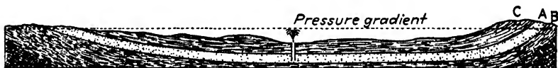
FIG. 132.—Ideal section illustrating the chief requisite conditions of artesian wells. A, pervious stratum; B and C, impervious strata. (After Chamberlin.)
