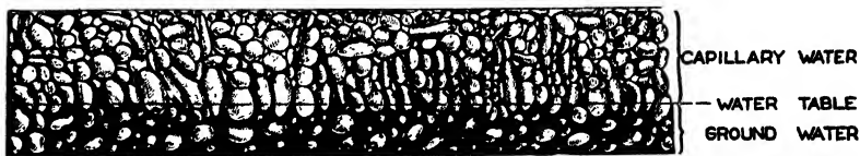
FIG. 5.—The capillary fringe. Capillary interstices near the base of the fringe are saturated; ground air appears in increasing amounts toward the top of fringe.
