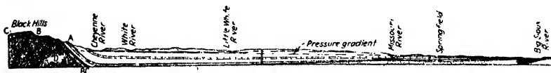
FIG. 134.—Geologic section across South Dakota. A, Dakota sandstone; B, Deadwood sandstone; C, Carboniferous limestone; D, schist. Pressure gradient shown by dashed line through section. (Modified after Darton.)
