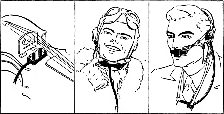
FIG. 12-2.—Contact-type microphones. (a) For musical instruments, (b) throat microphone, (c) lip microphone.
