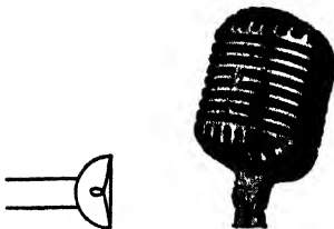
Dynamic microphone. (Moving coil.)
