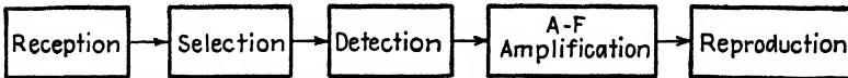
FIG. 14-3.—Block diagram of a simple receiver with the addition of a-f amplification.
