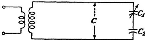
FIG. 6-9.—Increasing the frequency range of a tuned circuit by use of a fixed capacitor.
