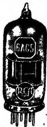
FIG. 4-39.—Miniature type tube with a button base. (Courtesy of RCA Manufacturing Co., Inc.)
