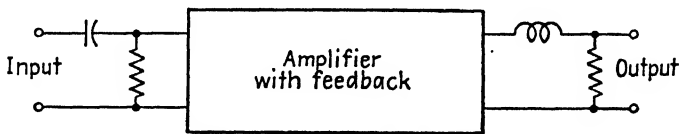
FIG. 8-24.—A feedback amplifier with equalizing filter networks for neutralizing the amplification peaks.
