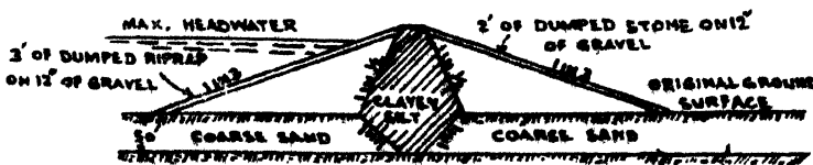
Fig. 6. Suitable design for a site where both clayey silt and coarse sand are available and where foundation is pervious for depth of 50 ft.
