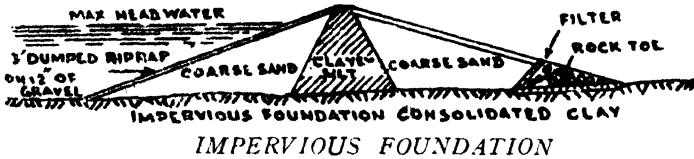
Fig. 7. Suitable design for a site where both clayey silt and coarse sand are available and where the foundation is impervious. Hence to prepare for this condition and avoid the possibility of sloughing due to saturation a rock toe with a filter consisting of smaller stones with gravel and sand just ahead of it to protect it against impregnation is utilized. Even without going into the design from a quantitative standpoint, it is evident that seepage will be entirely insignificant.
