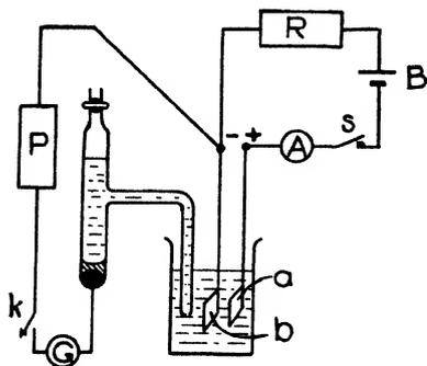
FIG. 9. Apparatus of Dutoit and von Weisse. *b*, cathodically polarized platinum electrode; *a*, auxiliary platinum electrode. The polarizing current was generally about  $1 \times 10^{-4}$  amp. maintained constant with the aid of battery, B, resistance, R, ammeter, A, and switch, S. P represents a potentiometer, G, a galvanometer.
