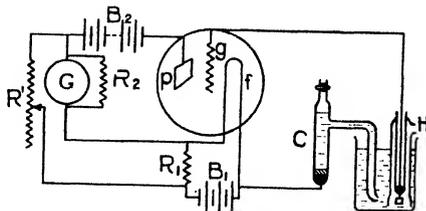
FIG. 15. Goode's Continuous Reading Electro-Titration Apparatus. C, calomel cell, H, hydrogen electrode, B<sub>1</sub>, six volt battery, B<sub>2</sub>, 22.5 volt battery, R<sub>1</sub>, resistance, about 0.6 ohm. R<sub>2</sub>, 25 ohms. R', variable high resistance. G, galvanometer. p, f, g, plate, filament, and grid of electron tube.
