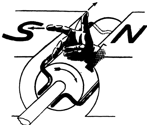
Fig. 32 Fleming's Rule for Generators.
