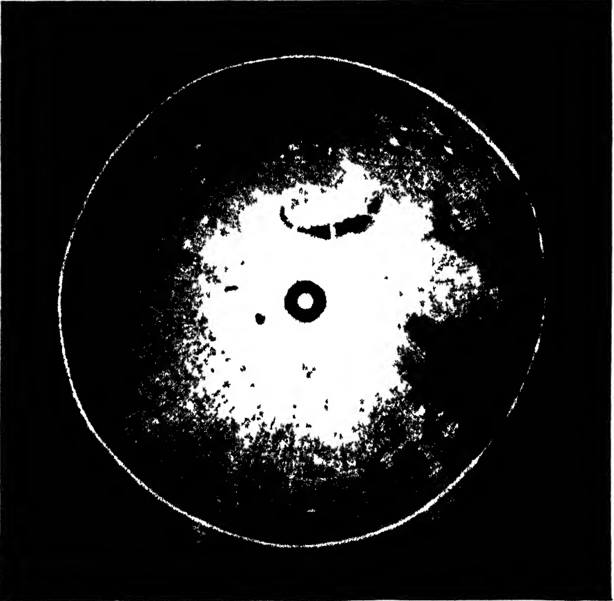
FIG 3 27—Boston, Mass., with "three-tone" presentation (Sec 13 21) Wavelength = 3.2 cm, 3° beam, altitude 4000 ft, radius 5 nautical mi 42°20'N 71°05'W.
