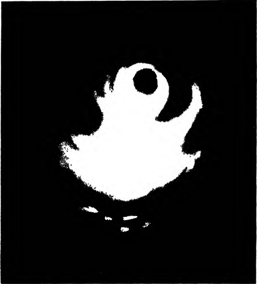
FIG. 3-12.—Echoes from a typhoon on the scope of a 10-cm shipborne radar system. "Eye" of storm is clearly visible above center of scope.
