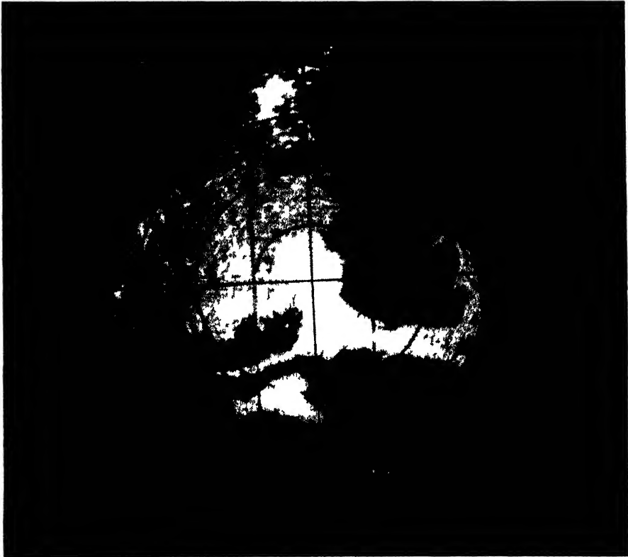
FIG. 9-9 — Photograph of PPI scope of 3-cm airborne radar: Cape Cod area
