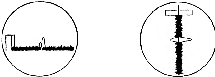
(a) Side-by-side presentation (K-scope). Signal return from the right lobe is the stronger. (b) Back-to-back presentation (L-scope). Signal return from the right lobe is the stronger.
