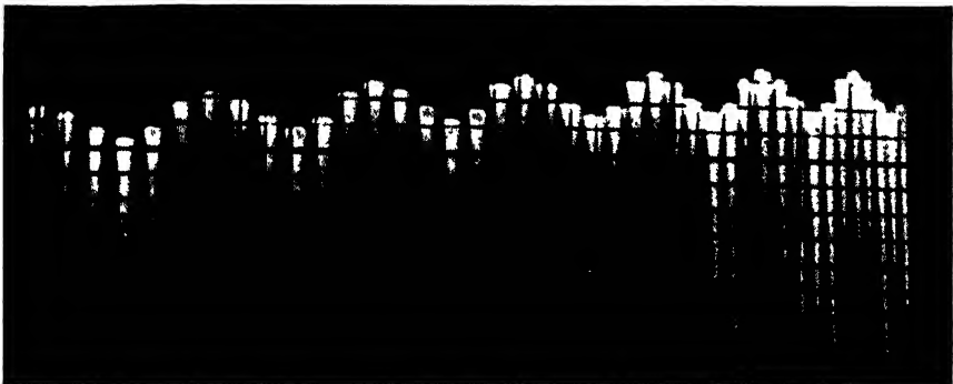
FIG. 14-11.—Output waveform showing amplitude modulation.
