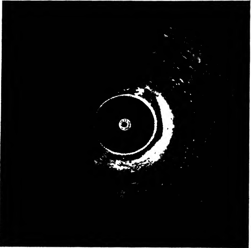
FIG. 3-31.—Kanazawa, Honshu. Wavelength = 3.2 cm, 3° beam, altitude 10,000 ft, radius 10 nautical mi. 36°40'N. 136°46'E.
