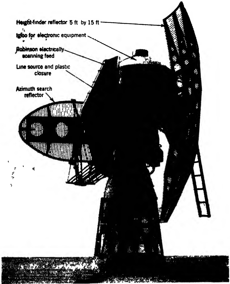
FIG. 9-28 —The three-axis antenna mount of the SGI radar.
