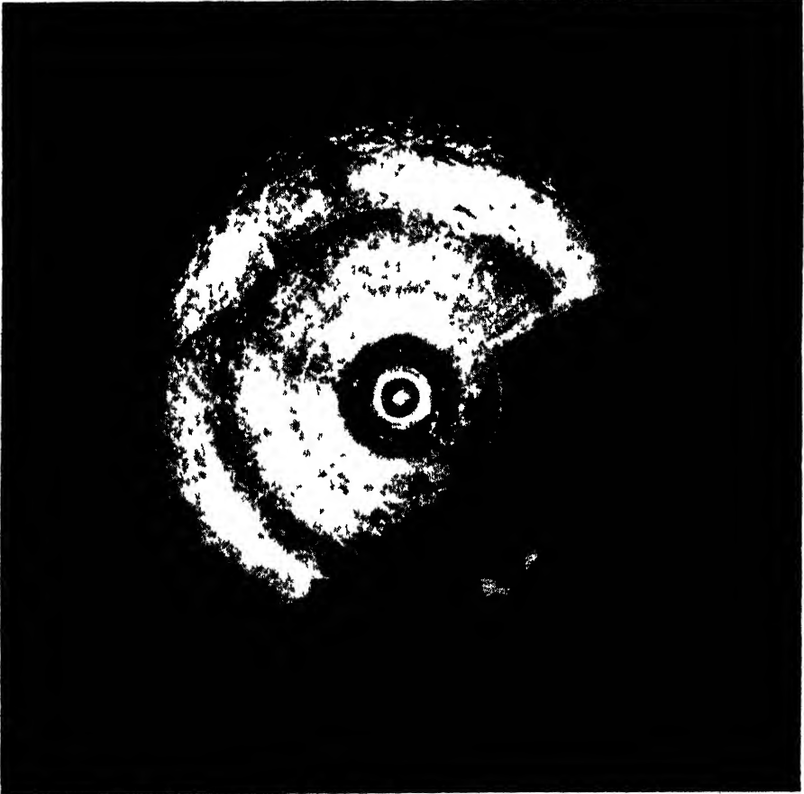
FIG 3-39—Pacific Coast near Balboa, C.Z. Average water-vapor concentration over flight path 6.9 \text{ g/m}^3 . Wavelength = 1.25 cm, 0.8^\circ beam, altitude 20,000 ft, radius 23 nautical mi. 9^\circ 01' \text{N} , 79^\circ 35' \text{W}
