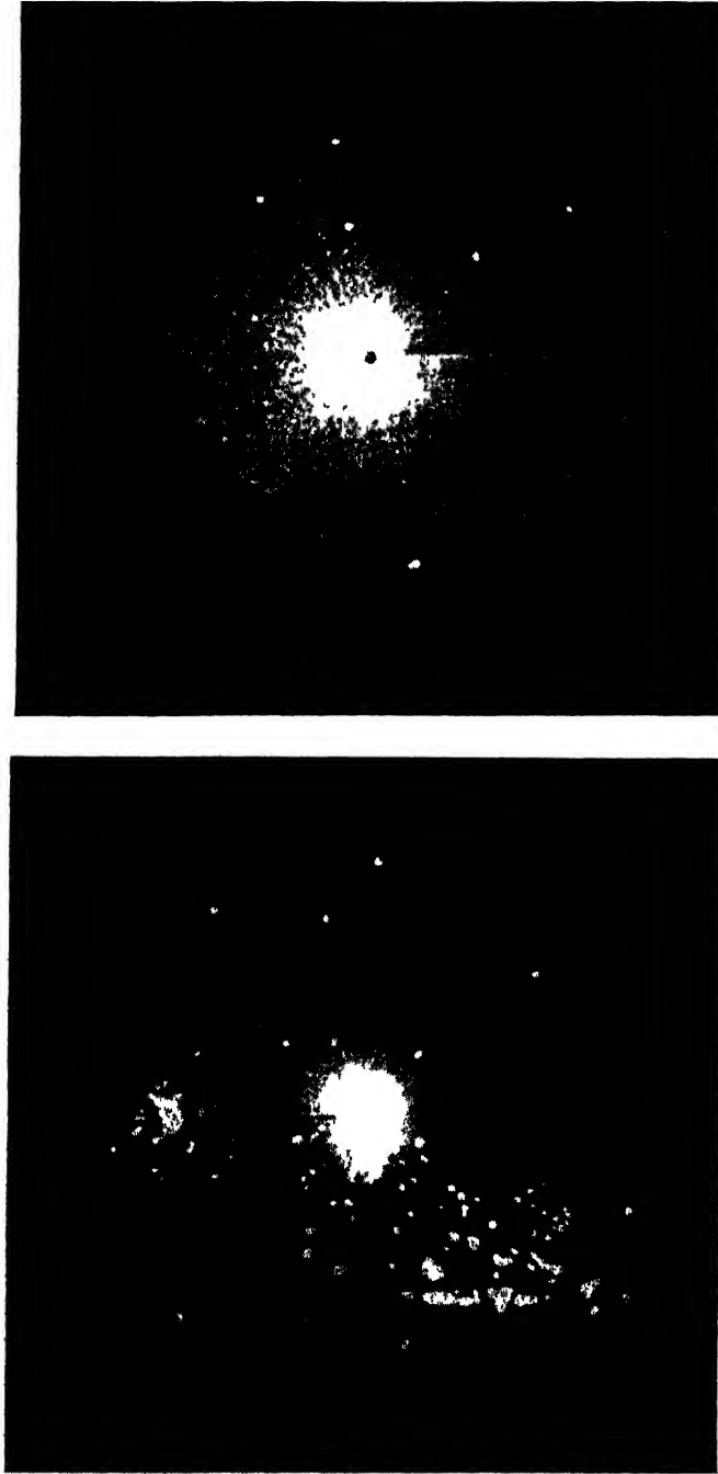
(a) (b) FIG. 16-1.—Comparison of normal and MTI PPI presentations: (a) normal scope, 35-mile sweep; (b) scope with MTI, 35-mile sweep.
