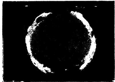
Fig. 229. Cross section of rod with coarsely crystalline peripheral zone.
