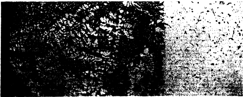
Fig. 130. Segregation of copper on casting in a cast iron mould \times 25 .
