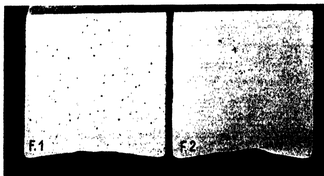
Fig. 105. (F. 1) Gas absorption by aluminium in new crucible. (F. 2) Gas-free metal from crucible preheated to redness for 16 hours.
