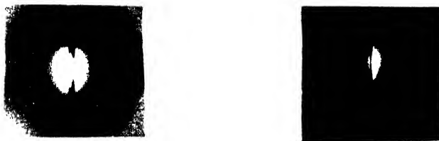
Fig. 49. X-ray low angle scattering of cellulose filaments imbibed with a) ethyl iodide, b) water
