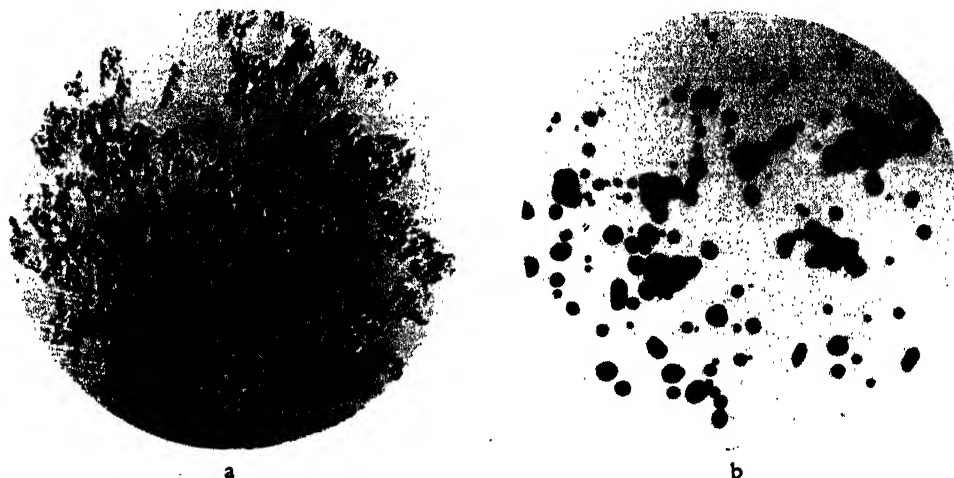
Fig. 6. Flocculation or coacervation with Na nucleate + hexol nitrate.
