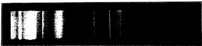
FIG. 18.-- Absorption spectrum of Li (principal series) according to Trumphy. The dark absorption lines crowd together towards the series limit on the right. The bright lines are emission lines of Mg.
