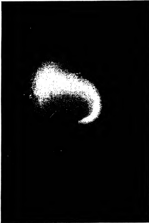
FIG. 2B.—Circular or spiral motion (as the case may be) of electrons in the magnetic field of a bar magnet MM.
