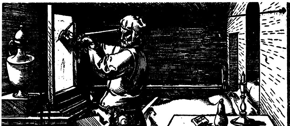
81 The productions of Albrecht Dürer, whose life-work vindicated the new style, illustrate explicitly the artistic investigation and discovery of his time. This Dürer wood-cut of 1525 shows a glass screen and levelling instrument used as aids to perspective drawing.
