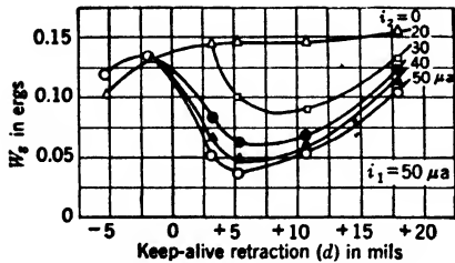
FIG. 6-18.—Spike leakage energy vs. distance of coaxial keep-alive electrode from the end of the cone in a 3-cm bandpass TR tube.
