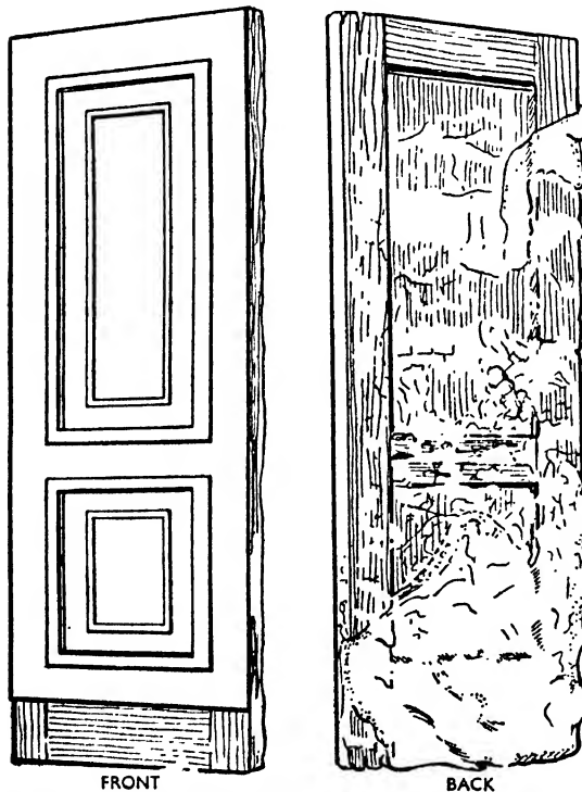
Fig. 3. Typical example of hidden decay in a portion of panelling. From the front view (left) the panelling appears to be quite sound but examination of the back (right) reveals the extraordinary extent of the decay caused by the wood-destroying fungal growth.
