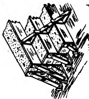
VERY MUCH ENLARGED VIEW SHOWING THE CELLS OF AND STRUCTURE OF A SOFT WOOD
