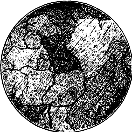
FIG. 11. PURE IRON ( \times 333 ). CRYSTALS OF FERRITE (PURE IRON) ONLY. NO CARBON
