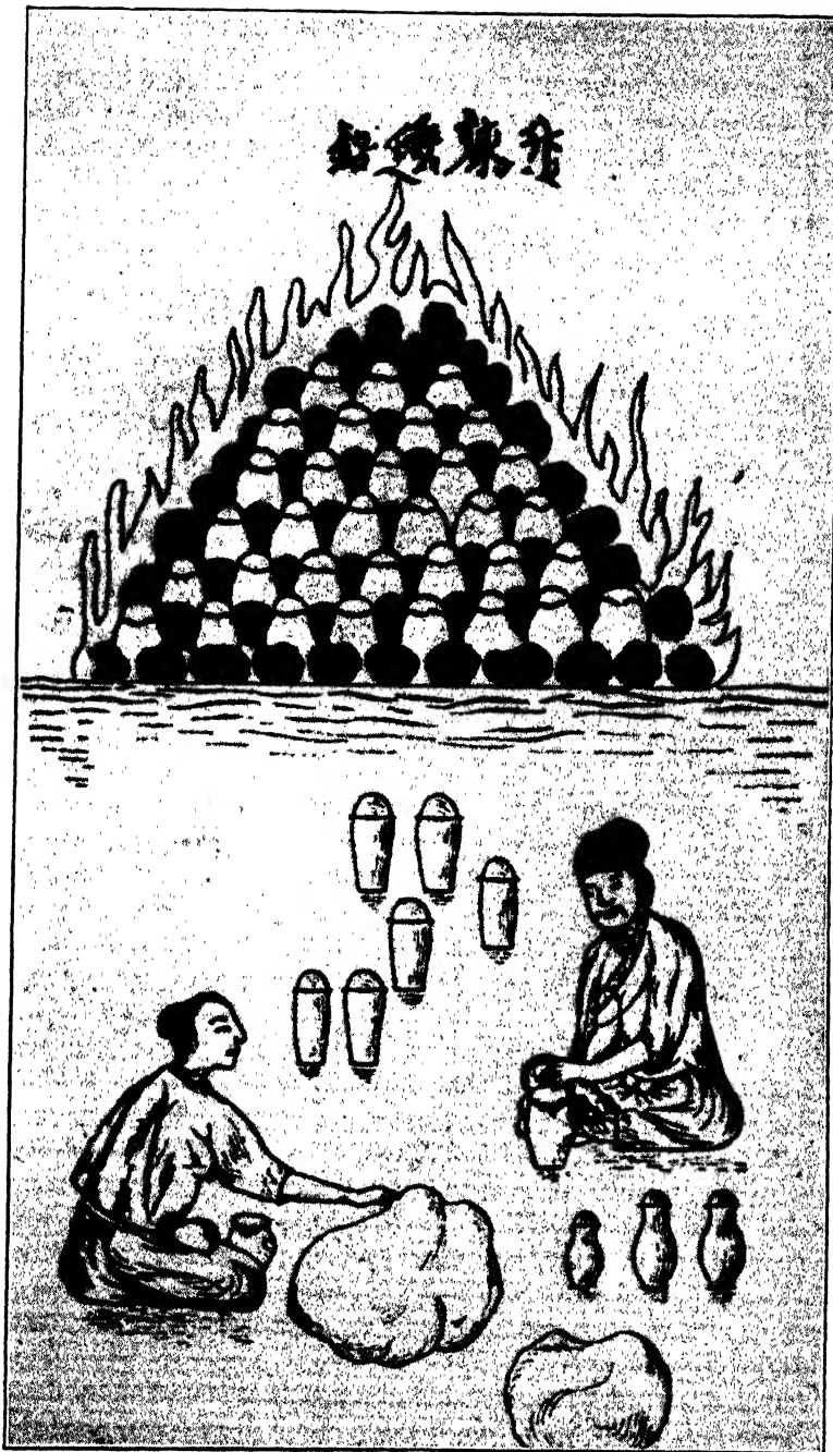
Z. Angew. Chem., 1912 Production of Zinc in China as pictured in the Chinese technical lexicon "Tien kong kai ou."
