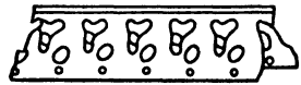
Fig. 85.—Corner bead provides a definite edge against which to finish the plaster. It also helps to form more accurately the shape of doors and other openings.
