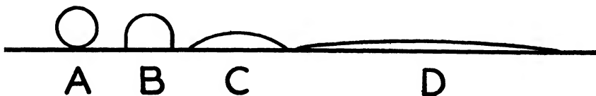
FIG. 26. Droplet forms illustrating different degrees of wetting and spreading.
