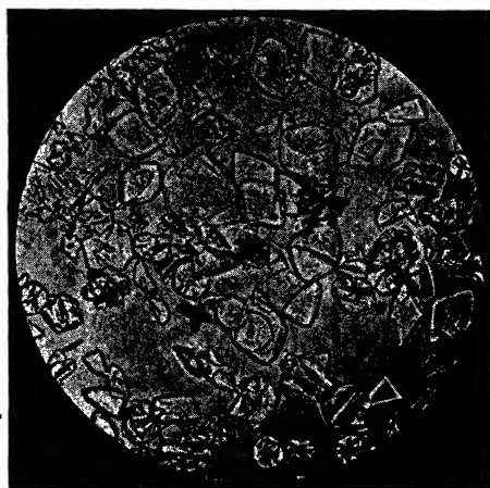
FIG. 17. Dimorphic form of dihydro-rotenone, m.p. 216^{\circ}\text{C.} 60\times . (Courtesy Dr. C. M. Smith.)
