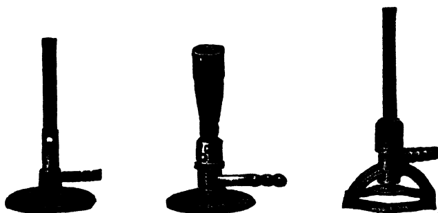
Fig. 147. The Bunsen, Meker, and Tirrill types of atmospheric gas burners. ( Courtesy of Eimer and Amend. )
