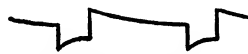
FIG. 8-19.—Typical wave form of condenser current or suppressor voltage for the circuit of Fig. 8-18.
