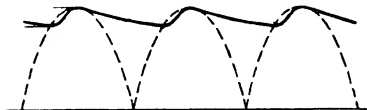
FIG. 11-5.—Wave form (solid line) of the condenser and load voltage in the circuit of Fig. 11-4a under light load.
