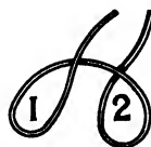
FIG. 47.—To complete the clove hitch the second loop is passed in front of the first.
