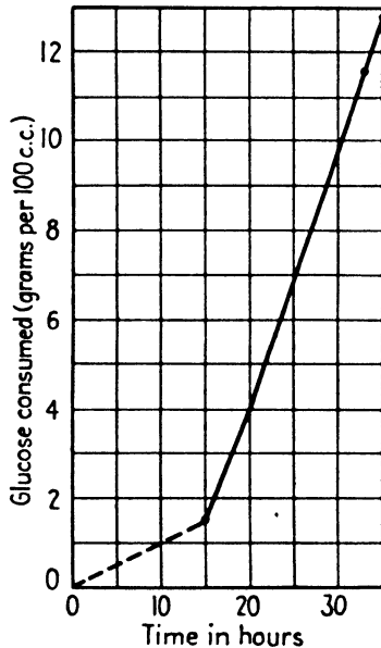
FIG. 48.—Course of a typical d -lactic acid submerged fermentation induced by Rhizopus oryzae . [Ward, Lockwood, Tabenkin, and Wells, Ind. Eng. Chem. , 30 : 1233 (1938).]
