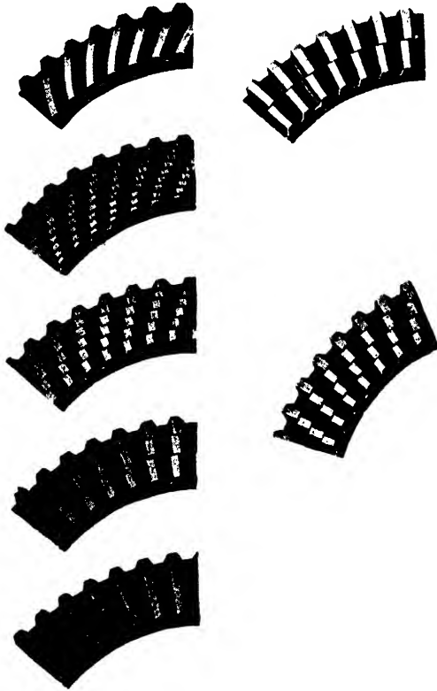
FIG. 4A.—How a number of sections of a straight-tooth bevel gear can be made to secure the action of a spiral bevel gear.
