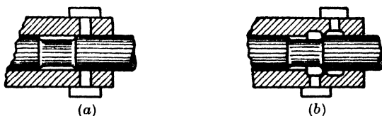
FIG. 47. PORT ARRANGEMENTS WITH SLIDE SELECTOR (a) = Unbalanced. (b) = Balanced.
