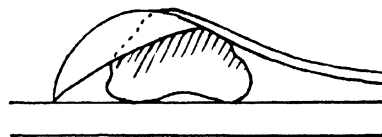
Fig. 12 Position of spoon for soldering
