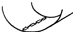
Fig. 11 Panels of solder placed along the seam
