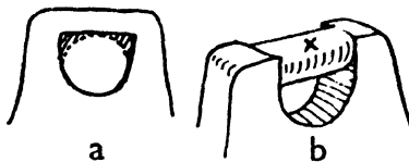
Fig. 10 (a) Shaping the hole for the loop (b) Shape of top of handle
